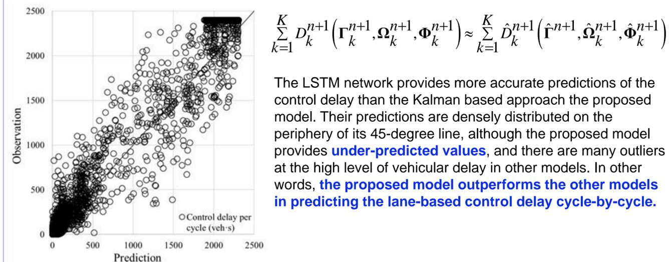
The LSTM network provides more accurate predictions of the control delay than the Kalman based approach the proposed model. Their predictions are densely distributed on the periphery of its 45-degree line, although the proposed model provides **under-predicted values**, and there are many outliers at the high level of vehicular delay in other models. In other words, **the proposed model outperforms the other models in predicting the lane-based control delay cycle-by-cycle**.
