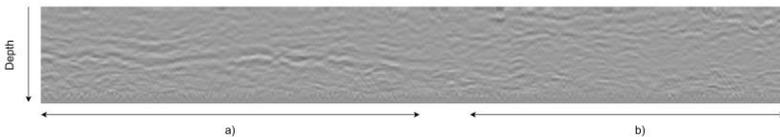
Figure 1: An example of GPR signal data, a) highlights a rare area of GPR data with a somewhat clear transition line with visual amplitude spikes, and b) depicts a more common area where there is no obvious transition line.
