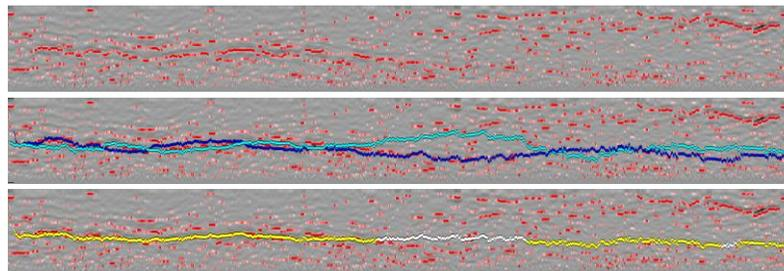
Figure 3: The three steps of the GRE algorithm. First, non-visual peaks are identified and ordered via prominence. Second, forwards and backwards passes are used to chain peaks together using a gaussian distributed weighted voting system creating an approximated transition line. Finally, the two approximated transition line are compared, with different features being generated based upon if the two lines differ greatly at a specific point (white), or if they are similar (yellow).
